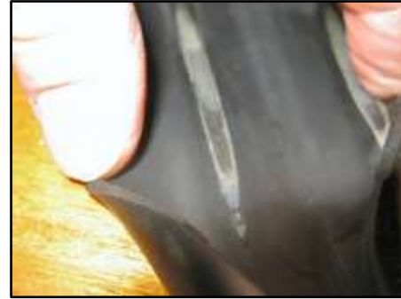
Fig. 8. Liner cracks with bacteria
