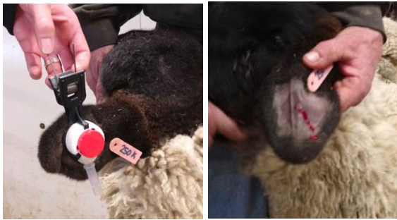
Figure 2.4: Tasso device tested on ear with clip. The picture on the right shows the blood flowing from the ear after the clip was removed. Vacuum and suction of blood into the tube is a problem. Ear and tail locations were tested with issues at both sites.
